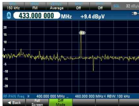
Difference spectrum in PScan with signal at 433 MHz
