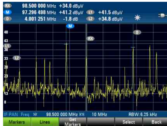
Marker functions within the IF spectrum display
